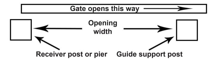
If you are installing new posts we would suggest 75mm -100 mm square as a good size and if concreting into the ground a minimum of 600mm in concrete with legs attached.
