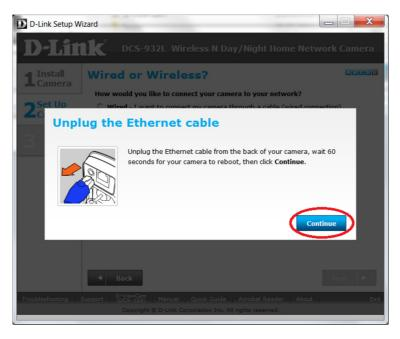
NOTE: When disconnecting the Ethernet cable, the power LED will turn Red to Reboot, once rebooted it should turn back to green. After 60 seconds has passed, now click on the Continue button.
