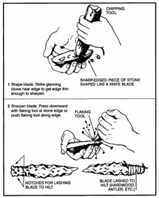
Figure 12-3. Making a stone knife.
