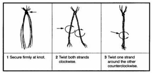
Figure 12-8. Making lines from plant fibers.
