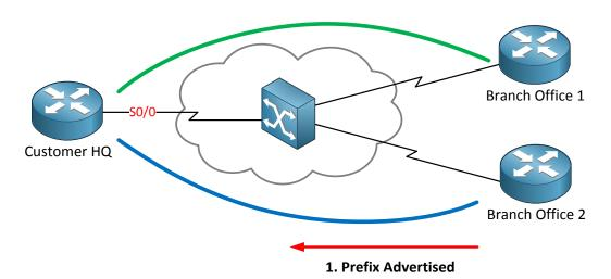
What other problems might we encounter with frame-relay and routing? Do you remember the characteristics of distance vector routing protocols (RIP and EIGRP)? Split-horizon anyone?
