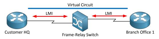
Here's an example of LMI in action. In the middle we have the frame-relay switch. LMI packets are sent between Router A and the frame-relay switch and router B and the frame-relay switch. The frame-relay switch tells our routers that the PVC is active.
