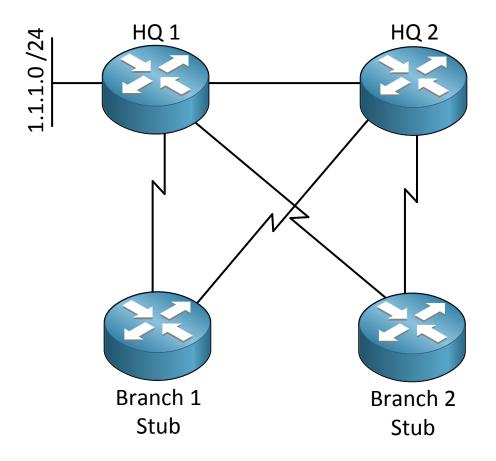
Look at the following topology. We have a company with a headquarters and 2 branch offices. The 2 HQ routers are connected on the LAN using a Gigabit link. The branch offices are connected to both HQ routers using slow 64kbps serial links. What do you think will happen once HQ 1 loses its route to the 1.1.1.0 /24 network on the left side?
