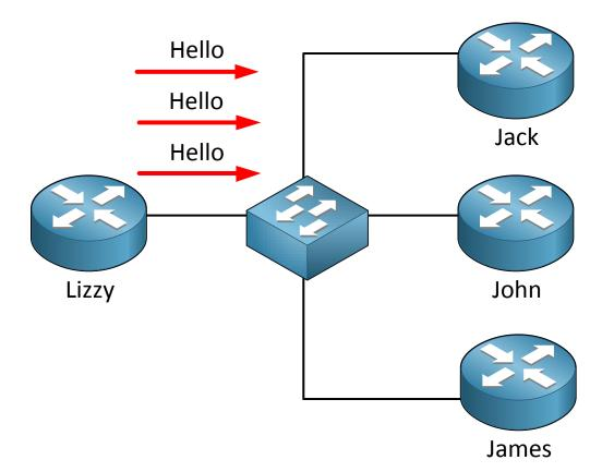
In this example we have 4 routers all running EIGRP. Hello packets are sent between routers in order to form adjacencies. As you can see router Lizzy is sending 3 hello packets meant for router Jack, John and Lizzy.
