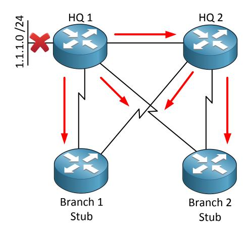
Query packets (red arrows) will fly everywhere! It doesn't sound like a good idea to use the serial links for backup so we are going to change this behavior by turning the branche routers into **EIGRP stubs**.
