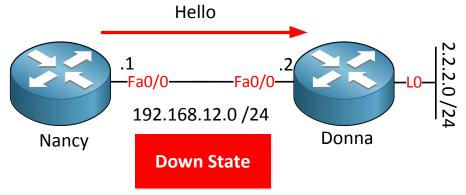
As soon as I configure OSPF on router Nancy it will start sending hello packets. Router Nancy has no clue about other OSPF routers at this moment so it's in the **down state**. The hello packet will be sent to the **multicast address 224.0.0.5**.
