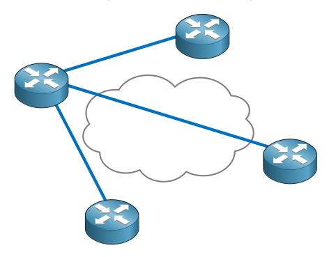
This is the hub and spoke model. The router on the left is our hub and the other routers are spokes. If the spokes want to communicate with each other they'll have to send traffic
