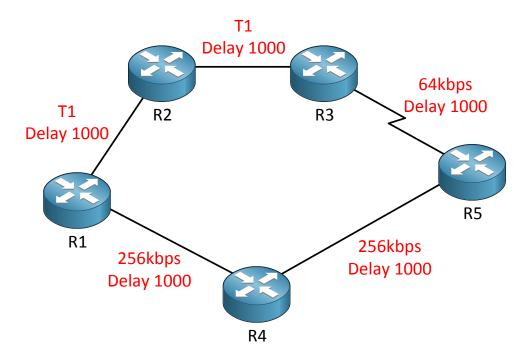
We are looking at R1 and calculating the distance to get to R5. As you can see there is an upper path with some T1 interfaces and a 64kbps link. The path below has two 256kbps links.
