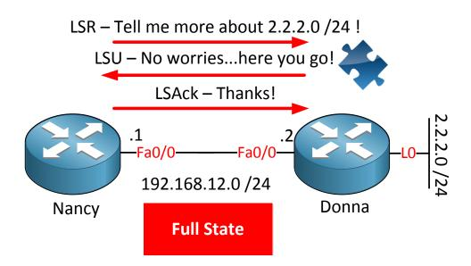
When router Nancy requested information about 2.2.2.0 /24 it used a LSR. Router Donna will send the LSU with the information. Router Nancy will send an acknowledgment using a LSAck packet to finish. We are now in the **full state.** Both routers have a synchronized LSDB and we are ready to route!
