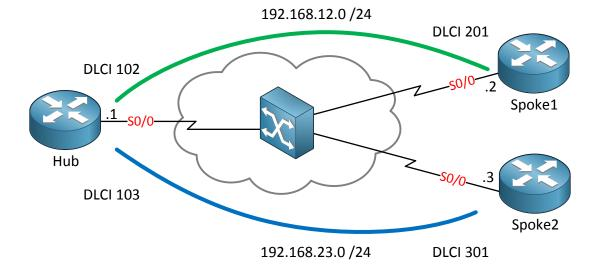
We are using the same topology to demonstrate point-to-point EIGRP over frame-relay with one difference. Point-to-point links require an **IP Subnet per PVC**:
