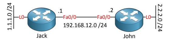
This is the topology I'm going to use to configure EIGRP. My goal is to have full connectivity and here are the configurations:
