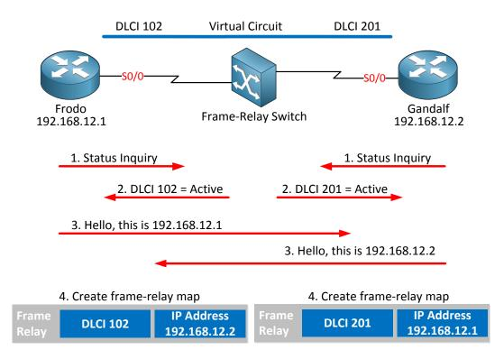
Router Frodo will now know it can reach IP address 192.168.12.2 by sending traffic through the PVC with DLCI 102. Router Gandalf will know that it can reach IP address 192.168.12.1 through the PVC with DLCI 201.
