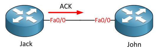
4. After both routers have exchanged hello packets we will establish the neighbor adjacency. Router Jack will send an ACK to let John know he received the update packets. The routing information in the update packets will be saved in the EIGRP topology table.
