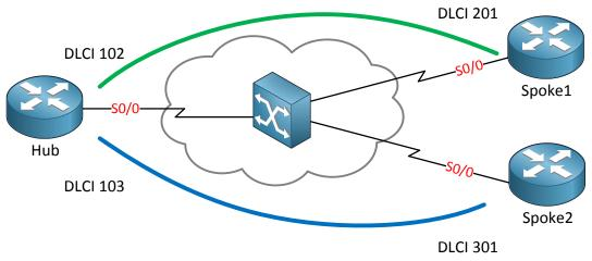
The topology above is the one I'm going to use to show you how to run EIGRP over a frame-relay network. On the left side we have a hub router and on the ight side 2 spoke routers. This is a classic example of a hub and spoke model and ideal for a lab.
