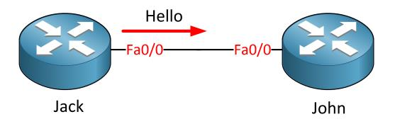
1. We have 2 routers called Jack and John and they are configured for EIGRP. As soon as we enable it for the interface they will start sending hello packets. In this example router Jack is the first router to send a hello packet.
