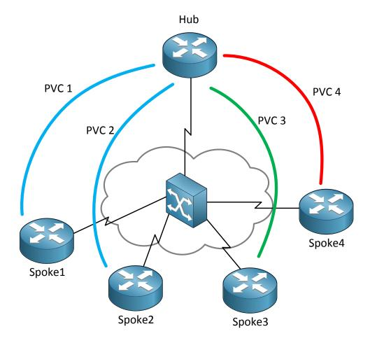
In the example above I have 5 routers in a hub and spoke model. The router on top is our hub and I have 4 spoke routers at the bottom. For each spoke there is a PVC and they each have a different CIR:
