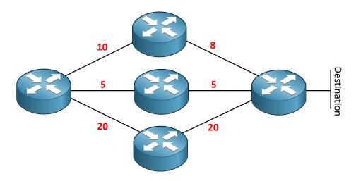
Look at the picture above, we are sitting in the router on the left and running the SPF algorithm looking for the shortest path to our destination. Which one are we going to use?
