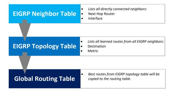
Instead of using just a single routing table EIGRP will use multiple tables. The first one is the **neighbor table** and this is where EIGRP stores all information of directly connected
