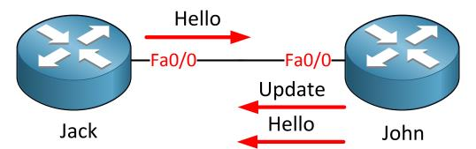
3. Router Jack is of course not the only one sending hello packets. As soon as router John sends a hello packet to Jack we can continue to setup a neighbor adjacency.
