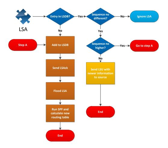
Each LSA has an **aging timer** which carries the **link-state age field.** By default each OSPF LSA is only valid for **30 minutes.** If the LSA expires then the router that created the LSA will resend the LSA and increase the **sequence number**.
