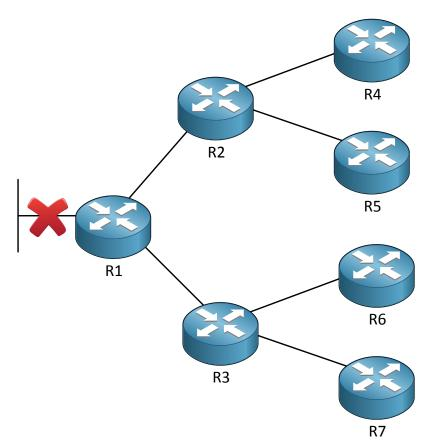
In the topology above we are running EIGRP on all of the routers. Router 1 has a link failure
