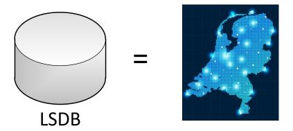
Once every router has a complete map we can start calculating the shortest path to all the different destinations by using the **shortest-path first (SPF) algorithm**. The BEST information goes into the routing table. Calculating the shortest path is like using your navigation system, it will look at the map and look at all the different ways of getting to the destination and only show you the best way of getting there.
