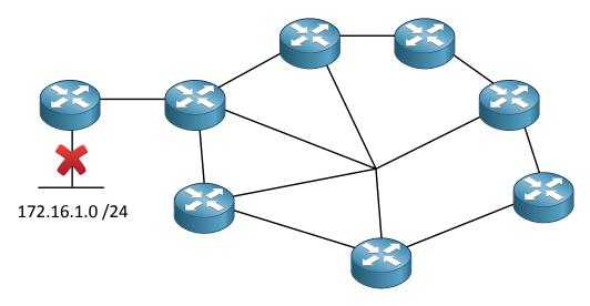
Look at the topology above. We are running EIGRP on all routers. The router on the left side has an interface that's going down.
