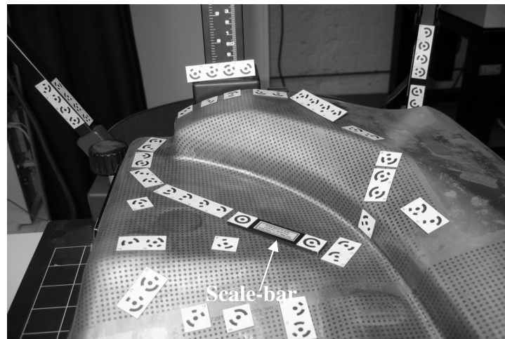
Fig. 6 Example of how the markers could be placed. Note that the markers do not have to be directly on the object's surface.
