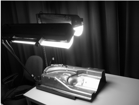
Fig. 7a Illumination setup. Creating diffuse light by using paper.
