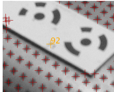
Fig. 10b Marker does not exist and must be deleted.
