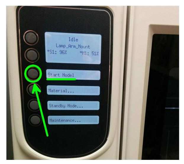
The printer's screen should show Idle status and the name of the print job you sent. Press the button next to "Start Model." That's it! The machine may take several minutes to warm up and calibrate before it begins printing. Check back in about 30 minutes to see how your print is going.
