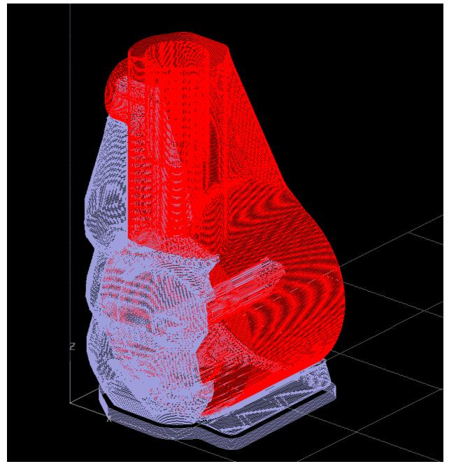
The software will slice the model into layers. Red lines indicate model material to be printed, while white lines indicate the soluble support material, which will later be dissolved away in a sodium hydroxide solution.
