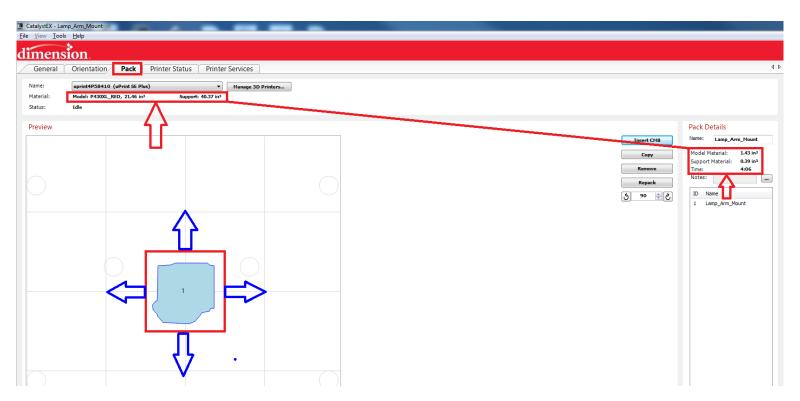
On the Pack tab, click and drag the model into position on the build plate. If you are using a build plate that has been used before, be sure to position the model on an area of the build plate that has not been printed on before. Each square in this pack view is 2 inches by 2 inches.
