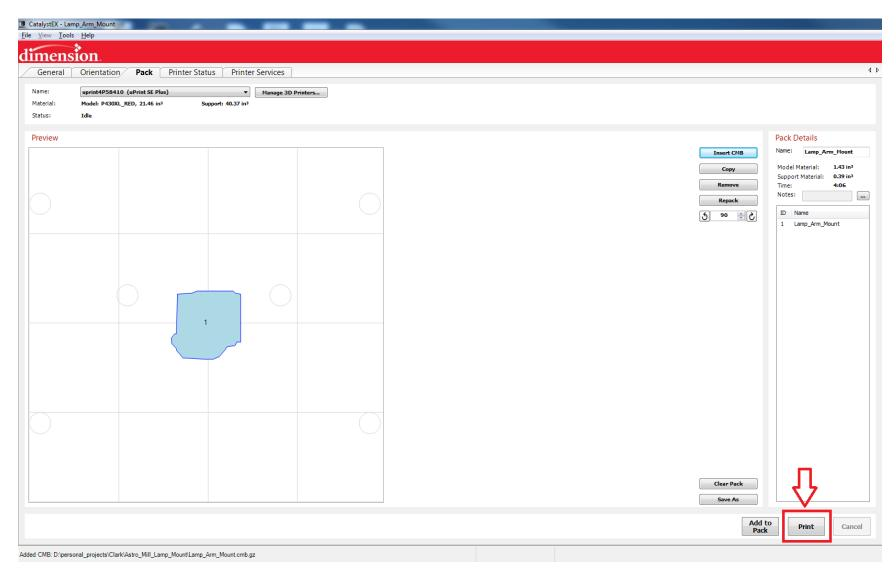
After verifying the model position on the build plate, the material consumption, and print time, click "Print" to send the pack to the printer.
