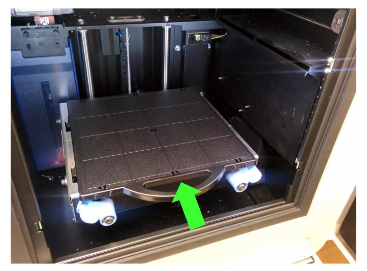
Insert a new build plate such that its tabs align with the cutouts in the top surface of the metal build table. Push it in fully until its front edge is flush with the front face of the metal build table.
