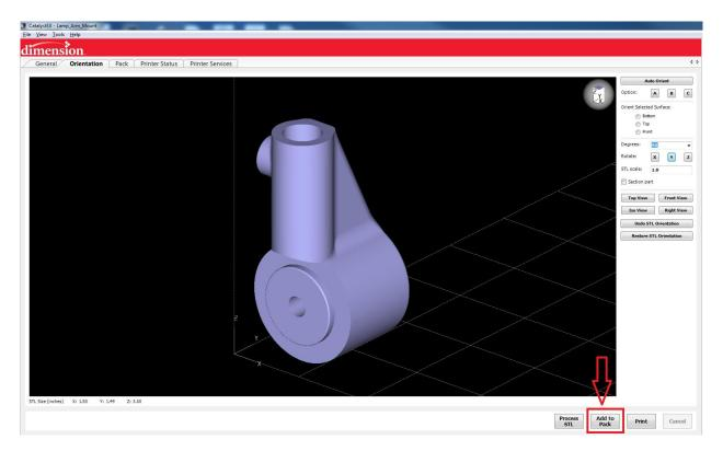
Once the scale has been verified, the type of model interior fill density has been set, and the desired orientation has been achieved, click the "Add to Pack" button.
