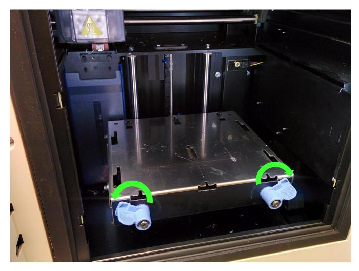
At the printer, open the blue thumb tabs so a new build plate may be installed.
