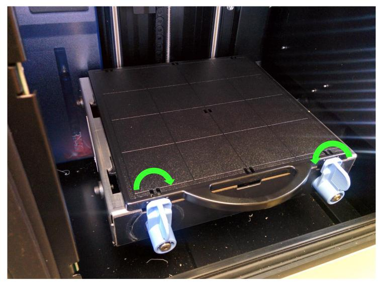
Rotate the blue thumb tabs to the vertical closed position as shown.
