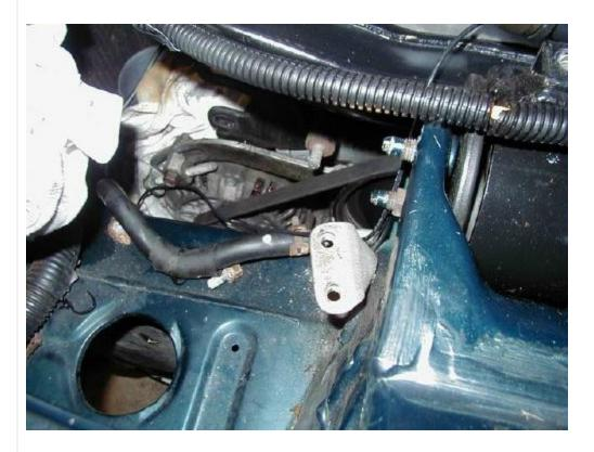
4. I removed the power steering cooling lines next, they are held on by 1 bolt that bolts into a vertical cross member behind the bumper. Assuming you don't have a FMIC they will be visible from the front.
