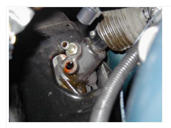
6. It's now time to remove the PS pump, since you will be eliminating the pump, you can go ahead and cut the belt off. The pump is held on to a bracket with 2 14mm bolts that can be accessed by putting a socket into the holes of the PS pump pulley. You may have to rotate the pulley to get to both of them. There is also a 1-wire connection going to the side of that, which must be removed. Once loose, the pump will wiggle itself out.
