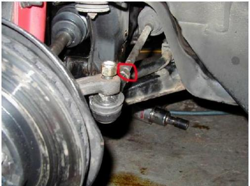
10. Once the tie rod ends are off, the last thing to do before you remove the rack mounts is to remove the bolt holding the steering shaft assembly to the steering rack gear box/spline.
