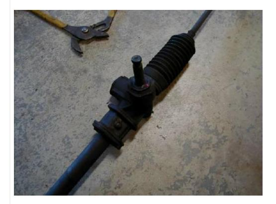
13. The manual rack will go in just like the PS rack came out. Remember you will need to use the new rack mount on the passenger side. You will see that the passenger side mount is a different shape for the PS rack then it is for the manual rack. Make sure the steering wheel is centered and you greased up the spline of the manual rack a bit, and then slide the rack in the same way.
