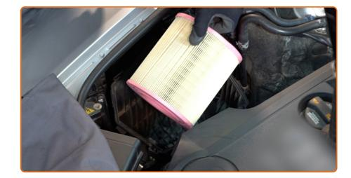
Remove the filter element from the filter housing.
