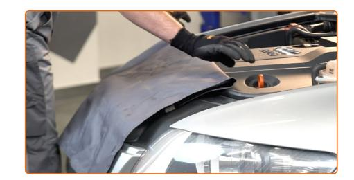
Use a fender protection cover to prevent damaging paintwork and plastic parts of the car.
