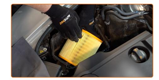
Insert a new filter element into the filter housing. Make sure that the filter edge fits tight to the housing.
