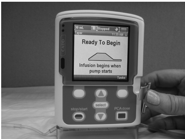
Lift the cassette handle into the closed position
