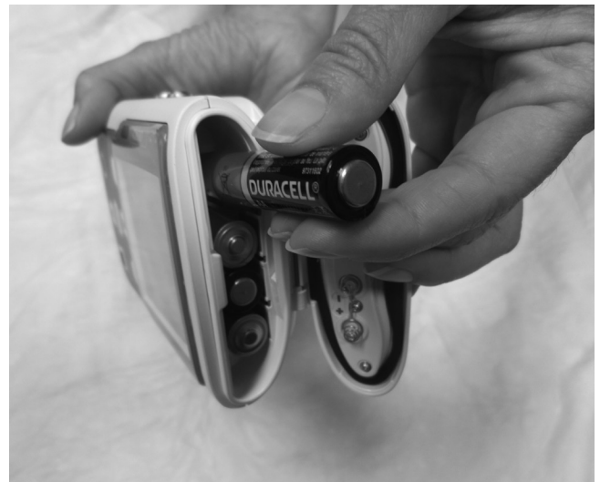
Insert AA batteries from the bottom up, matching the + and- markings
