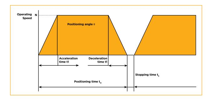
Last, calculate for the required torque, T, in Ib-in. The required torque is made up of the combination of the acceleration torque, T<sub>a</sub>, and the load torque, T<sub>L</sub>. First calculate the acceleration torque, T<sub>a</sub>. T<sub>a</sub>=  $((1.2J_L)/386)(V_m/(9.55t_1))(1/16)$ , where J<sub>L</sub> is the total system inertia, V<sub>m</sub> is speed of the motor, and t<sub>1</sub> is the acceleration /deceleration time.
