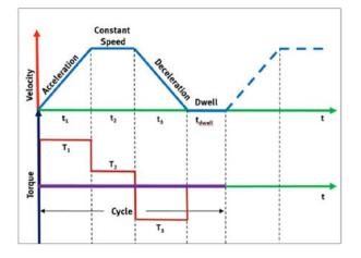
The servo motor's main feature is the capability to develop peak torque for 1-3 seconds, so for an indexing application the entire move is usually only acceleration/deceleration, with acceleration using the peak torque of the motor.
