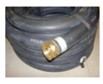
terial, by all means USE IT! Also black 5/8" water hose is fantastic, easy to connect and a great alternative but does not last as long (3 years). Ploy hose is designed for sub-
