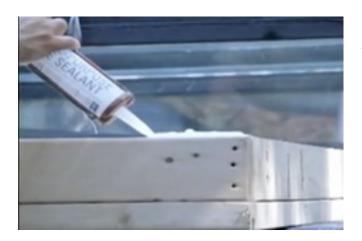
By simply searching for table tops with chipped corners, old unused glass doors or the best option, a double pained window as large as possible, you build a custom box out of 2x4s. This is simple framing cut to size, place silicone
