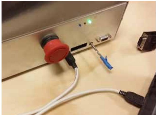
Step 9 – Turn ON the power to the control box. The green will flash a few times and then glow steady or go off completely. Either is OK. • If the green light doesn't flash when the controller is turned on, check the washer and magnet connections, and try again. If it still doesn't work, contact our Customer Support team for help (page 2).
