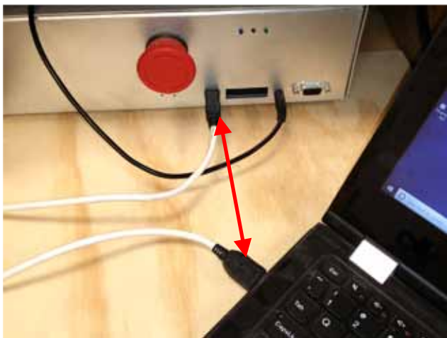
Step 6 – Connect your computer to the control box with a USB A/B (printer style) cable.
