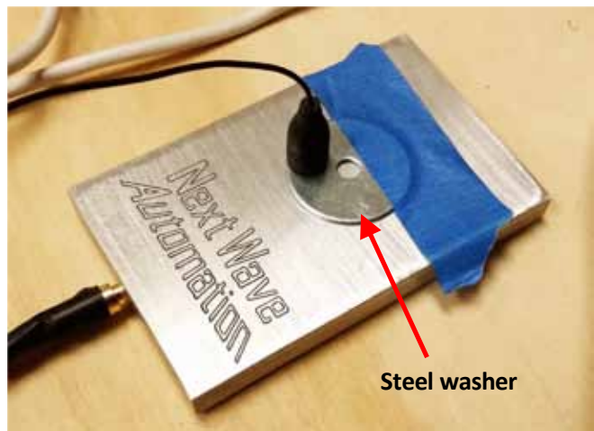
Step 7 – Tape a steel washer to your touch plate and attached the magnet to the washer. This connection is required when updating the firmware.
