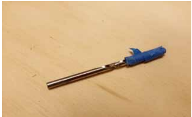
Step 7 – Put a piece of tape on the cutting end of a 1/8-in. dia. drill bit.
