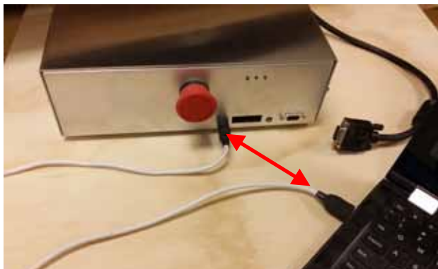
Step 6 – Connect your computer to the control box with a USB A/B (printer style) cable.
