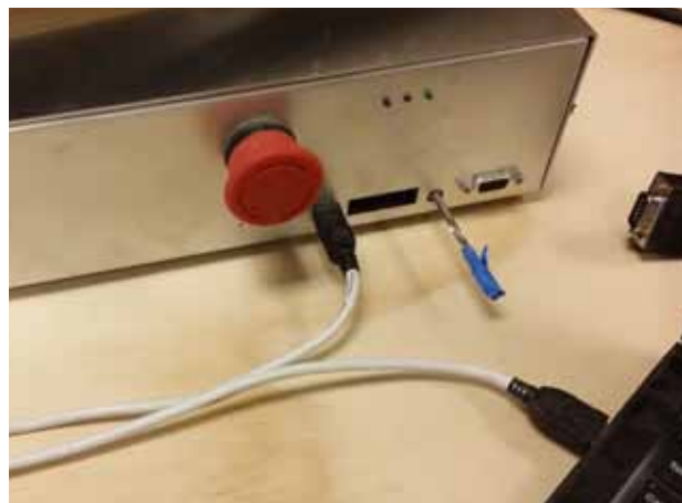
Step 8 – Insert the smooth end of the drill bit into the touch plate port.
