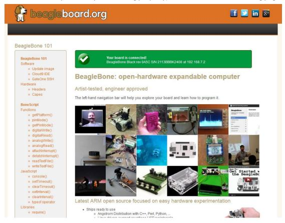
**Update on board Operation System**. (This step can be skipped) Download the latest software from <a href="http://beagleboard.org/latest-images">http://beagleboard.org/latest-images</a>. Unzip it and write the image to SD card. Insert SD card into Beaglebone Black, hold USER/BOOT button when start Beaglebone Black. Wait until all 4 LEDs be lit solid. It can take up to 45 mins. For more detail, go to <a href="http://beagleboard.org/Getting%20Started">http://beagleboard.org/Getting%20Started</a>.
