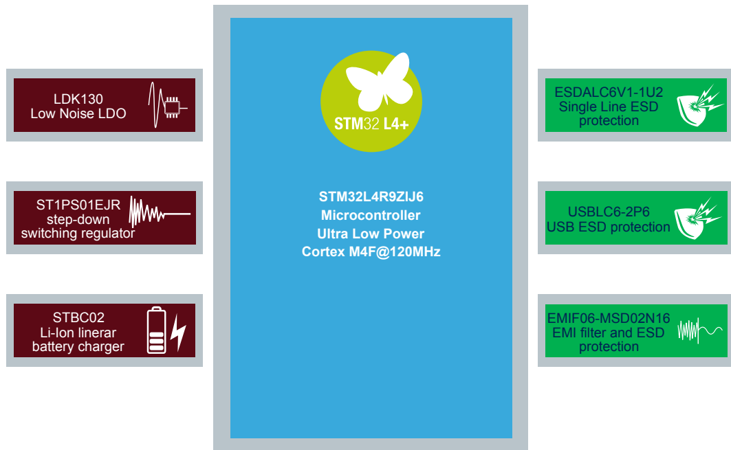
Figure 12. Power and protection components
