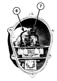
Step 4. Set multimeter for voltage check. Place red lead (8) in lamp socket, and black lead to ground, and check for 24 V dc.
