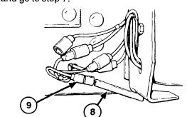
Step 6. Connect lead 461 or 460 (9) at rear harness connector, and disconnect lead 461 or 460 from lead 22 at intervehicular connector. Place red lead in lead 22 and check for 24 V dc.
