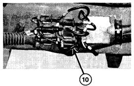
Step 7. Remove composite light assembly (para 4-23), and make sure mounting surface is clean.
