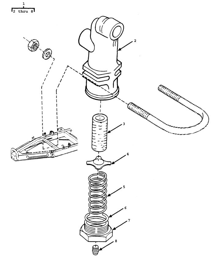
Figure 12. Air Line Filter Assembly
