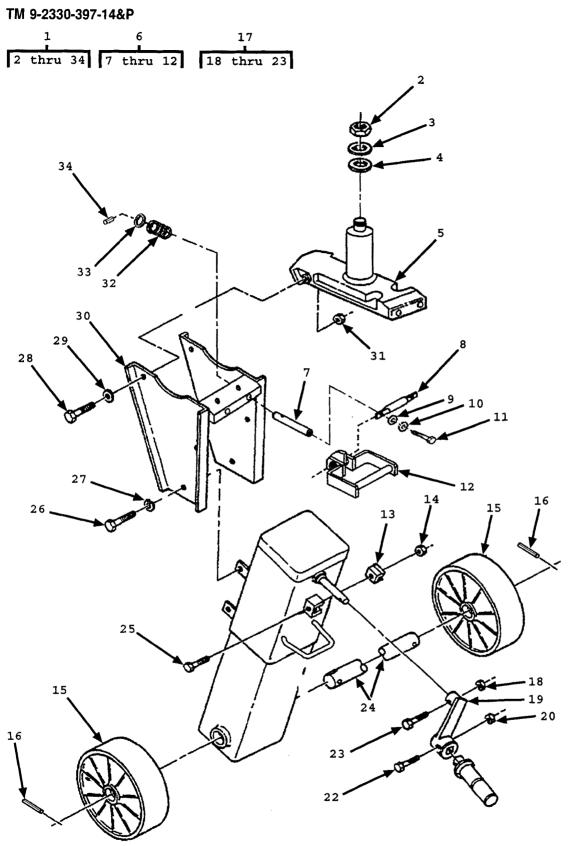
Figure 16. Caster Assembly, Folding Adjustable
