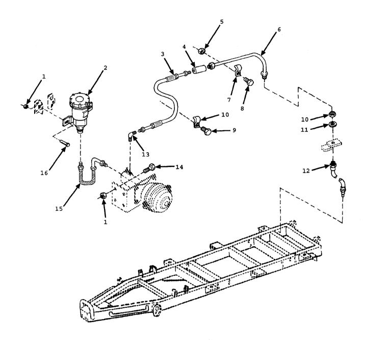
Figure 9. Front Hydraulic Brake Lines, Hoses, and Fittings
