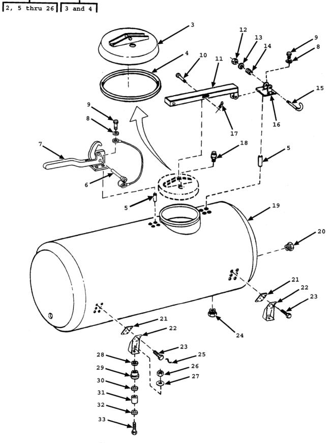
Figure 20. Tank Body (Without Heater)
