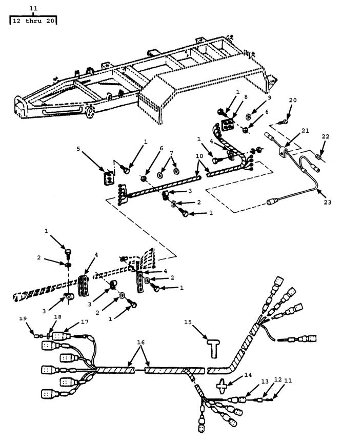
Figure 2. Chassis Wiring Harness
