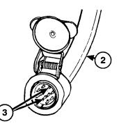
Step 3. Disconnect lead 489 from lead 21 at clearance light. Place red lead in lead 21, and black lead to ground, and check for 24 V dc.
