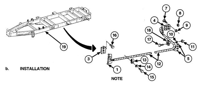
Perform Steps 1 and 2 only if brackets or retaining strap were removed.
