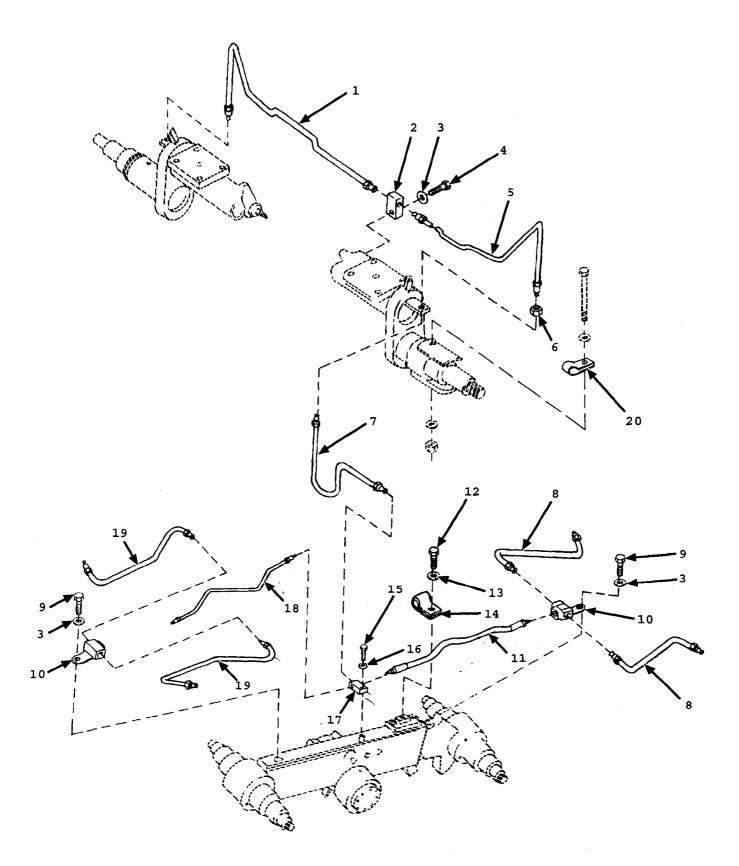
Figure 8. Rear Hydraulic Brake Lines, Hoses, and Fittings
