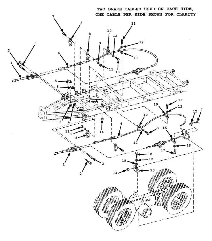
Figure 6. Handbrakes, Controls and Linkage
