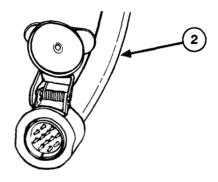
Step 7. Remove composite light assembly (para 4-23), and make sure mounting surface is clean.
