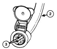
Step 2. Check intervehicular cable (2) for corrosion, frayed spots, cuts, and proper connection.
