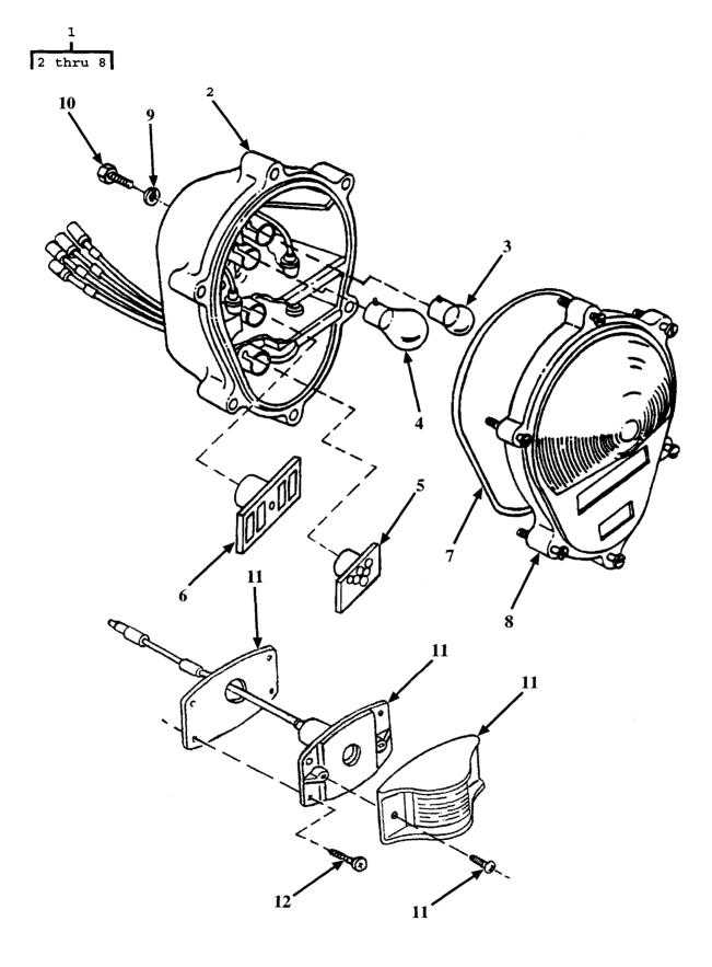
Figure 1. Composite Stoplight-Taillight
