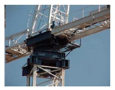
1) The long horizontal jib (or working arm), which is the portion of the crane that carries the load. A trolley runs along the jib to move the load in and out from the crane s center:
