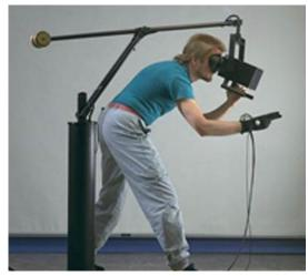
A BOOM Display used by NASA to emulate space Photo courtesy of NASA
