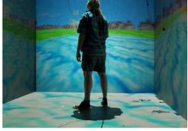
A virtual reality CAVE display projecting images onto the floor, walls and ceiling to provide full immersion. See more virtual reality pictures. Photo courtesy of Dave Pape
