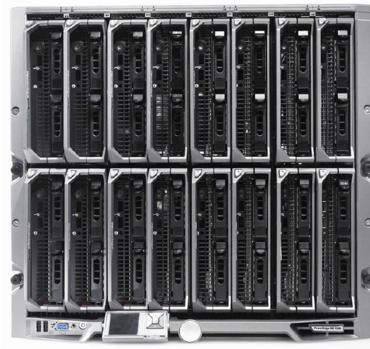
Figure 8. Dell PowerEdge M1000e Chassis and CMC (From Loffink, 2008)
