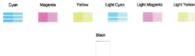
Figure 9-2 Example of color blocks with defects
