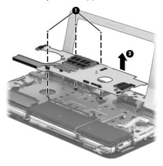
Reverse this procedure to install the system board.
