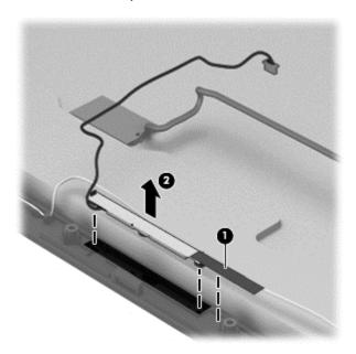
Reverse this procedure to install the webcam/microphone module.
