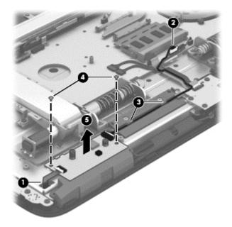
Reverse this procedure to install the converter board.
