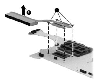
The thermal material must be thoroughly cleaned from the surfaces of the heat sink and the system board components each time the heat sink is removed. Replacement thermal material is included with the heat sink and system board spare part kits.
