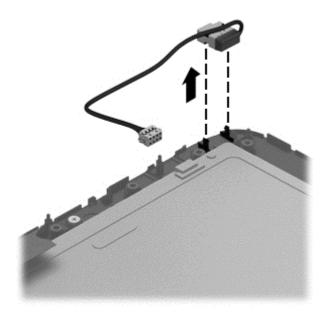
Reverse this procedure to install the power connector cable.
