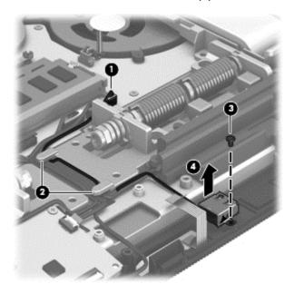
Reverse this procedure to install the USB connector cable.
