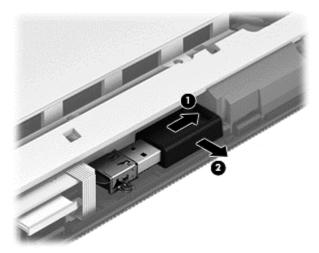
3. Insert the replacement dongle (1) into the cavity next to the internal USB connector.
