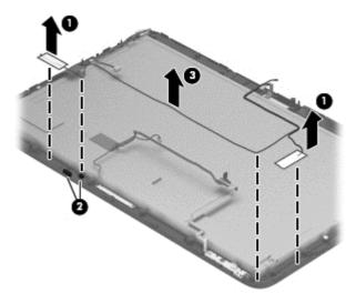
Reverse this procedure to install the wireless antenna.
