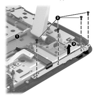
Reverse this procedure to install the audio/USB board.
