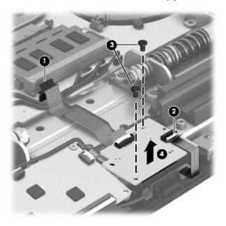
Reverse this procedure to install the media card reader board.
