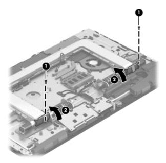
3. Press down on the display stand release actuator (1). (The display stand (2) releases to the open position.)
