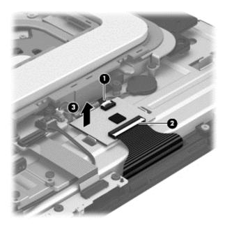
4. Remove the Y-axis capacitor board.
