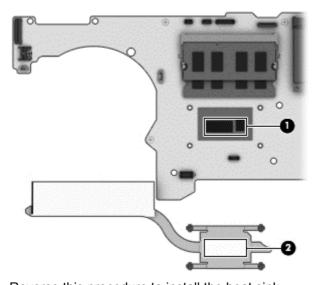
Reverse this procedure to install the heat sink.
