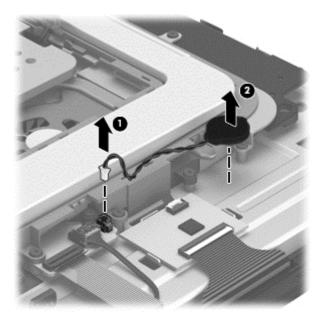
3. Remove the RTC battery.
