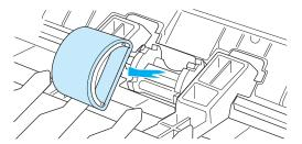
6 Position the new or cleaned part in the slot of the previous pickup roller. See <u>Cleaning the pickup roller</u> for instructions. Circular and rectangular pegs on each side prevent you from incorrectly positioning the pickup roller.
