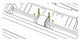
5. Gently pull the pickup roller up and out.
