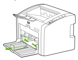
3. Place the envelopes with the side to be printed facing up and the top edge along the left media guide. Stack up to 15 envelopes.
