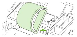
7. Rotate the top of the new pickup roller away from you until both sides snap into place.
