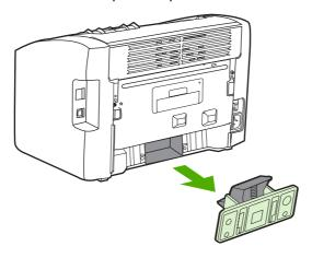
4. Insert the new separation pad, and screw it into place.
