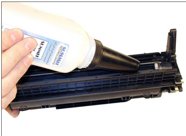
20. There is no fill hole in these cartridges so it must be filled through the DB slot. Fill the cartridge with 305g of P3005 toner. If a seal is available, install it now.
