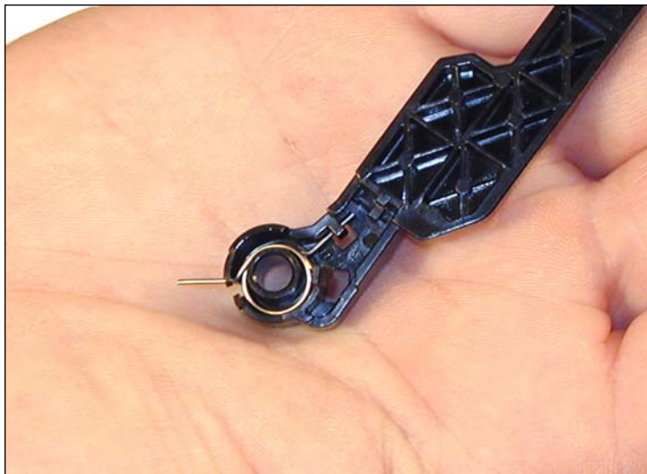
27. Install the spring in the drum cover arm as shown. Install the metal bar into the hole and slot. Install the arm.
