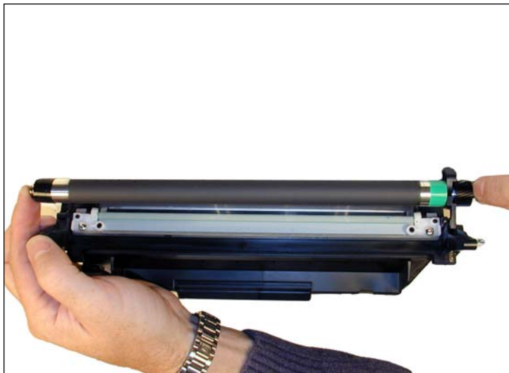
18. Remove the magnetic roller assembly from the cartridge.
