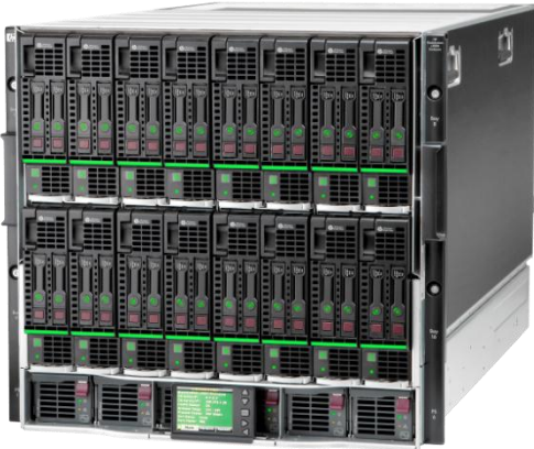
Figure 1: The HP BladeSystem c7000 enclosure (pictured with HP ProLiant BL460c Gen8 server blades)
