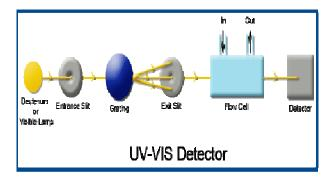
UV-VIS Detector is the most commonly used detector. Its response is specific to a particular compound or class of compounds depending on the presence of light absorbing functional groups of eluting molecules. Some compounds which do not have such light absorbing groups can give suitable response after post column derivatization to introduce light absorbing entities.
