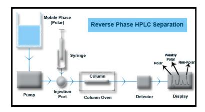
Majority of HPLC applications are covered under reversed phase chromatography. Stationary phases mostly comprise of non polar alkyl hydrocarbons such as C-8 or C-18 chains bound to Silica or other inert supports. C18 columns actually can handle more than 60% of the applications in most HPLC labs. Mobile phase is polar and the elusion order is polar followed by less polar and weakly polar or non-polar compounds in the end.
