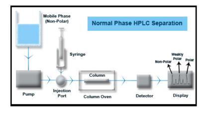
Normal Phase separations are the opposite of reverse phase separations. The stationary phases are polar having either plain silica or organic compounds such as amino, cyano, etc., groups bound to silica based supports. Mobile phases are non-polar such as hexane, heptane, etc. with
