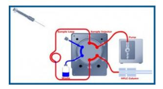
Injection is done through specially designed 6-port rotary injection valve. The sample is introduced at atmospheric pressure by a syringe into a constant volume loop. In the LOAD position the loop is not in the path of the mobile phase. By rotating to the INJECT position the
