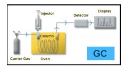
In Gas chromatography same principle is used but carrier is a gas instead of a liquid. The stationary phase is an immobilized liquid bound to an inert support or simply applied to the inner surface of a column. Gas chromatography is effectively used for analysis of gas mixtures or liquids having low boiling points. On the other hand liquid chromatography is applied for separation of thermally labile liquid mixtures or those having high boiling points.
