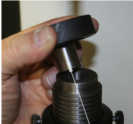
Insert anvil into up/down screw feed
