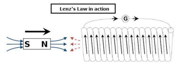
Using the right-hand GRIP rule (for coils) you can quickly and easily work out the direction of the induced current.
