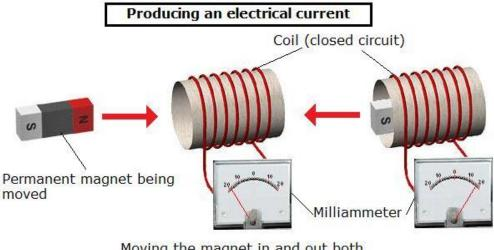
Moving the magnet in and out both generates a current, but in the opposite directions, as represented by opposite movements of the milliammeter.
