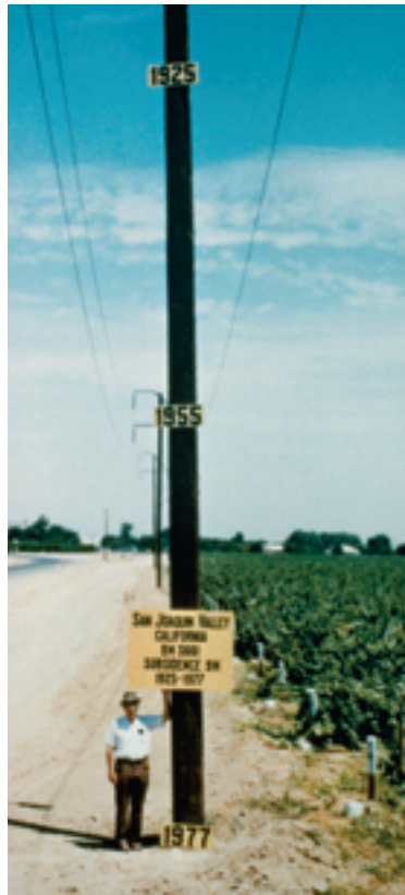
Figure 18 The marks on the utility pole indicate the level of the surrounding land in years past. Between 1925 and 1975 this part of the San Joaquin Valley sank almost 9 meters because of the withdrawal of groundwater and the resulting compaction of sediments.
