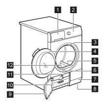
The load door can be installed by the user in the opposite side. It can help to easily put and remove the laundry or if there is a limit to install the appliance (see separate leaflet).
