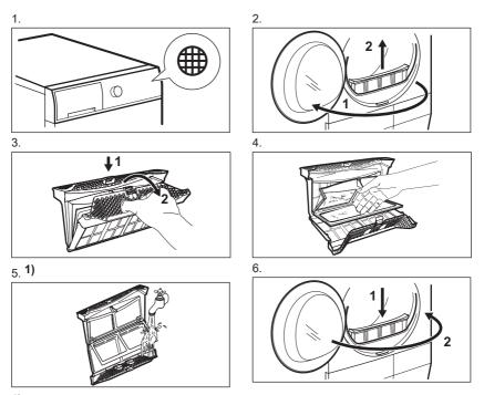
1) If necessary clean the filter with tap warm water using a brush and/or a vacuum cleaner.
