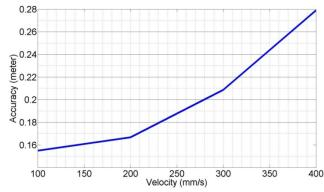
Figure 8: Sniffer Velocity VS. Localization Accuracy
