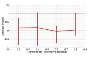
Figure 12: Transmission Time Interval VS. Localization Accuracy
