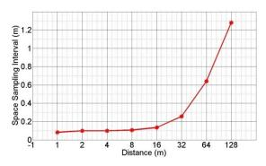
Figure 11: Space Sampling Interval VS. Estimated Target Distance
