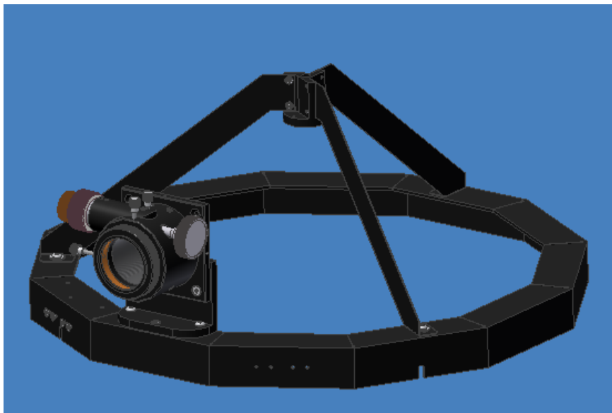
Figure 11: Attach the focuser to the L bracket
