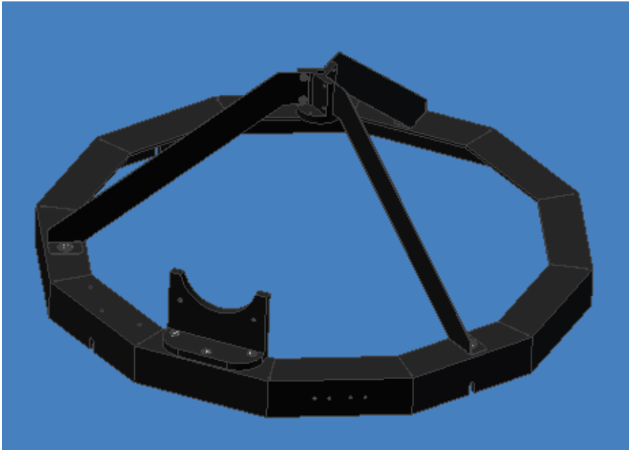
Figure 10: Attach the focuser L bracket to the upper ring
