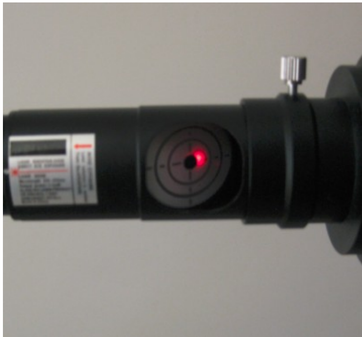
Figure 24: The primary mirror is not yet collimated.
