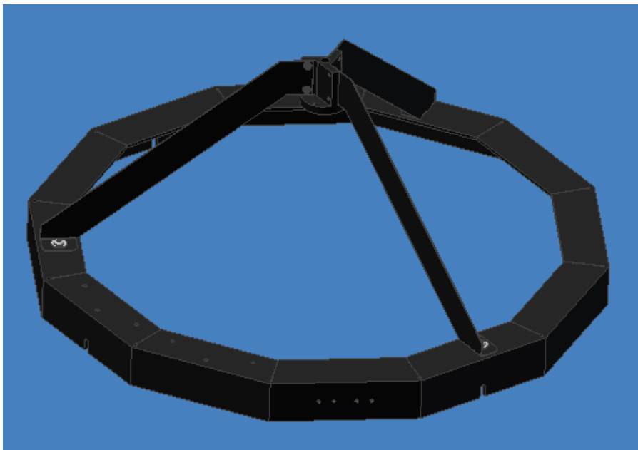
Figure 9: Attach the three spider wings to the upper ring
