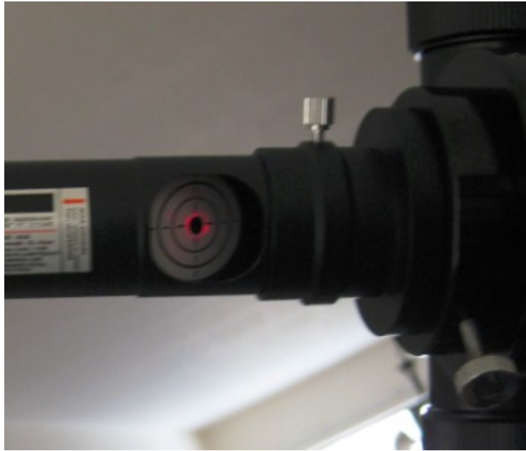
Figure 25: The primary mirror is collimated by laser collimator.
