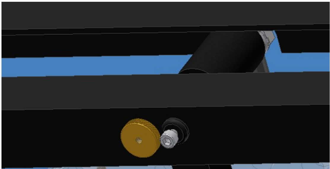
Figure 19: Primary Mirror Collimation Knob and Locking Screws
