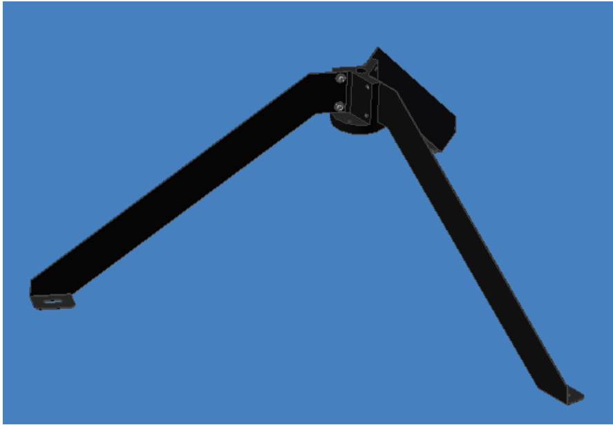
Figure 8: Attach the three spider wings to the spider hub
