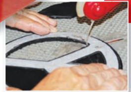
Make inside cuts! Separating blade in action.
