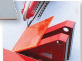
The magnetic tray angles make it possible to cut both 90° and 45° cuts.
