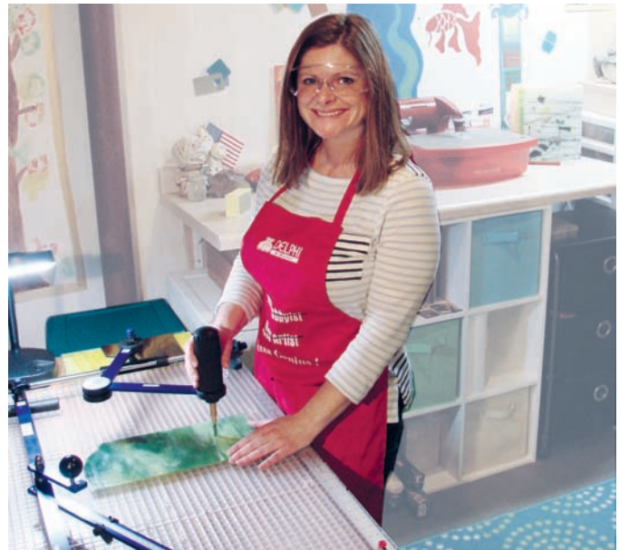
The foam cushioned, weighted handle eliminates the strain of grasping a cutter.
