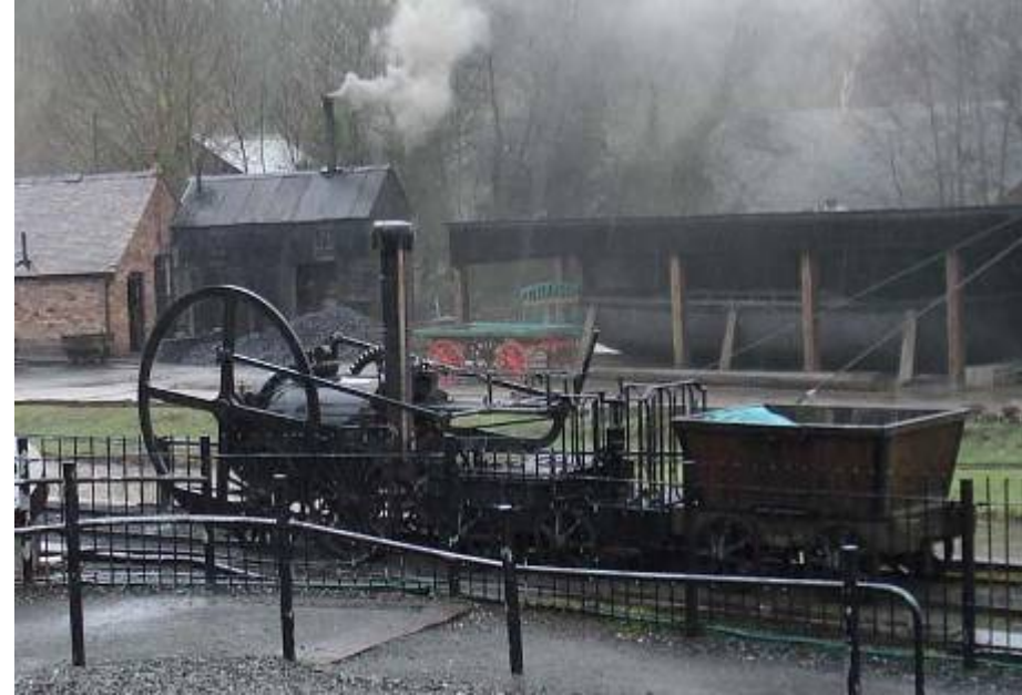
Trevithick's \frac{1}{2} scale model to test his high pressure engine for use as a rail locomotive. England about 1800.
