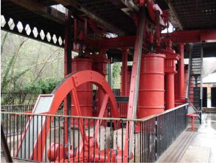
Watt's low pressure steam engine used to pump air into a blast furnace. England, about 1785
