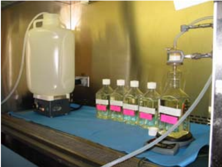
Fig. 1. Media filter sterilization setup inside laminar flowhood. Batch reagent reservoir on magnetic stirrer. Culture filter capsule, sterile media bottle, and digital scale.
