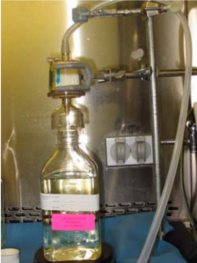
Fig. 3. Media capsule filtration into sterile 1-L bottles. Bottles filled by weight.
