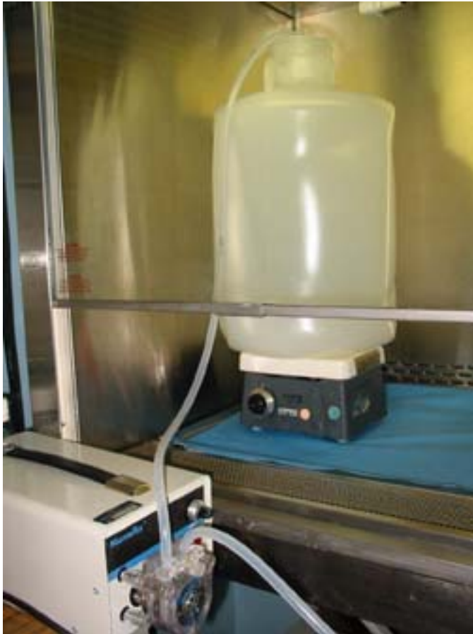
Fig. 2. Batch reagent reservoir and peristaltic drive pump for media filtration.
