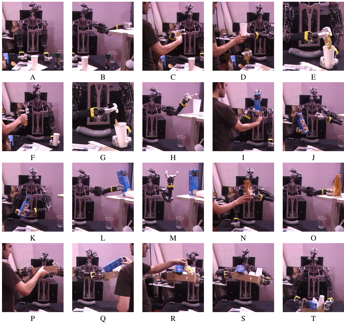
Fig. 7. In this sequence, Domo assists in a variety of manual tasks. (A) Domo begins at a cluttered table. (B) A shelf appears and Domo verifies its location. (C-D) A juice bottle and cup are handed to Domo. (E) Domo visually guides the bottle into the cup. (F-G) Now, Domo is handed a spoon and it “stirs” the drink. (H) Finally, Domo puts the finished drink on the shelf. (I-L) A box of crackers is handed to Domo’s right hand. It transfers them to the left hand and places them upright on the shelf. (N-O) A bag of coffee beans is handed to Domo. This time, it uses its left hand because of the person’s proximity. It then puts the bag on the shelf. (P) Domo forms a bimanual grasp on a box. (Q-R) Domo keeps the box near the person as they clean up the table and put items in the box. (S-T) Now that the task is done, Domo lowers the box onto the table
