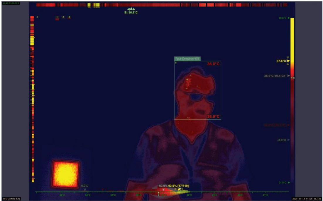
Figure 8.7: Preview of final user interface representation for history inspection (face detection history)
