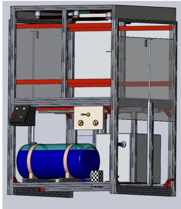
Figure 5: Solid Modeling of Boeing's current oven, the water tank, steam generator, controls mechanism and oven shell are detailed
