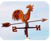
Wind direction is measured with a wind vane.
