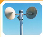
Wind speed is measured with an instrument called an anemometer.
