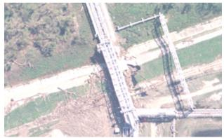
Figure 10. Mississippi River Levee Breach at ConocoPhillips Refinery during Katrina
