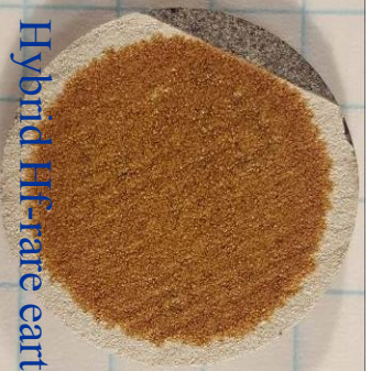
Special processed Yb 2 Si 2 O 7 , spalling at 450 Cycles
