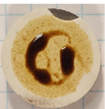
Plasma sprayed (Gd, Y) 2 Si 2 O 7 , 2450 cycles
