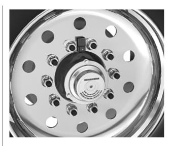
Figure 7: Properly installed WEM
