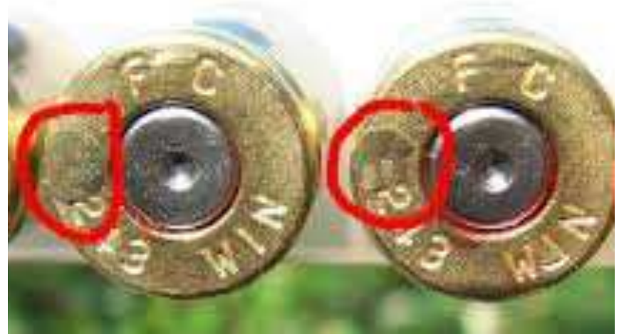
Extractor and Ejector Marks Cartridge Fired in Colt 45 Automatic Pistol
