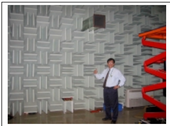
Figure 6 - McQuay's Anechoic Test Facility
