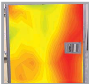
Vibration response test for side panel. Red/yellow indicates high levels of vibration.
