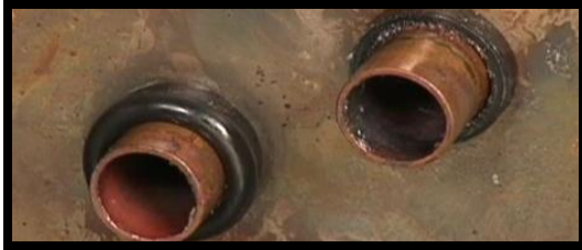
Annealed fins – Low Water Flow
