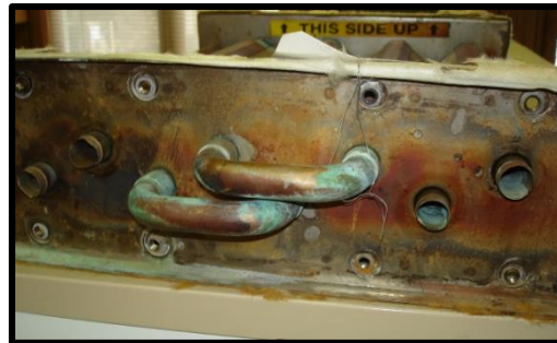
Sooted – Improper Fuel and Air Mixture.
