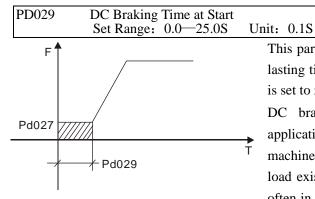
This parameter is set for DC Braking at start and the lasting time of DC Braking current to the motor. If it is set to zero it means DC braking is invalid.
