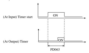
For example, set PD063=5.0s. When the external control terminal (Multi-Input) is valid the output terminal will be valid after five (5.0) seconds, the signal of which can be used to control other corresponding signals.
