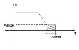
Note: When this parameter is set to any non-zero value it starts DC brake at stop and sends the DC braking time to the motor. DC braking at stop is often used for a high-level stop or positioning control. When this parameter is set to zero it closes DC braking at stop.
