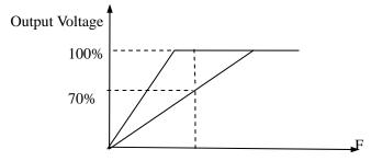
Auto energy saving can reduce the normal output voltage by max 30%. For the load with frequent changes or closing to full load, this function is not suitable.
