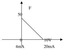
Note: this curve is a kind of special application of reverse ramp setting. When using transmitter for the control of pressure, temperature and others and while the control has higher pressure and output signals but requiring the corresponding commands of stop or deceleration on the inverter this curve can satisfy the demand properly.
