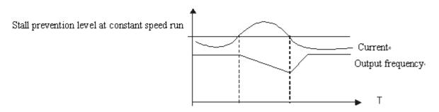
100% current is the Rated Current of the motor. When this parameter is set to 0 the stall prevention function is invalid.
