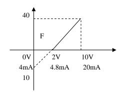
Note; this curve is the extension of the above curve.  $2V\sim10V$  (4.8mA $\sim20$ mA) corresponds to 0Hz $\sim40$ HZ; the signal of  $0V\sim2V$  (4 $\sim4.8$ mA) is invalid. It can be used to avoid noice disturbance. In harsh environment it is better not to use signals below 1V for setting the operating frequency of the inverter.
