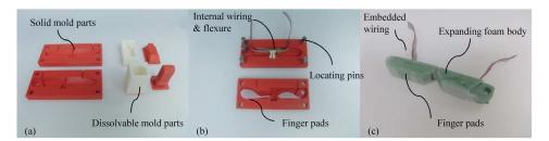
Fig. 10 Finger design where the proximal and distal digits are deposited around embedded components. (a) Multiple mold pieces are printed separately with both ABS and dissolvable material to facilitate the fabrication of urethane components, (b) internal components are positioned in the larger finger mold before the finger links cavities are filled with expanding foam to create the final product (c).
