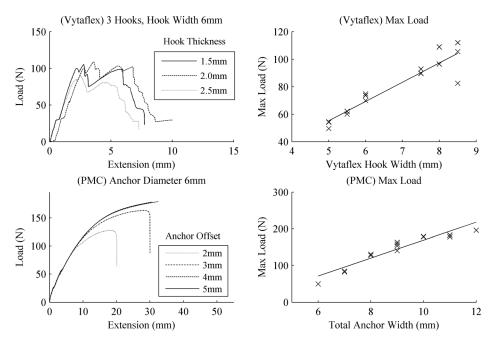
Fig. 4 Tensile test results to determine failure points of various anchor designs. Results suggest maximizing the overall resin anchor protrusion size.
