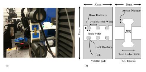
Fig. 3 (a) Instron setup to test the tensile strength of various resin anchors in combination with printed ABS bodies and (b) parameters of the test samples for both Vytaflex 30 pads and PMC-780 flexures
