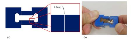
Fig. 6 Regions printed side by side as separate contours can produce dissolvable or breakaway molds. In this example, the 0.1 mm gap separation is guaranteed to be smaller than the standard FDM printer's nozzle diameter ( $\sim$ 0.4 mm). The optimal gap separation will depend on printer performance.
