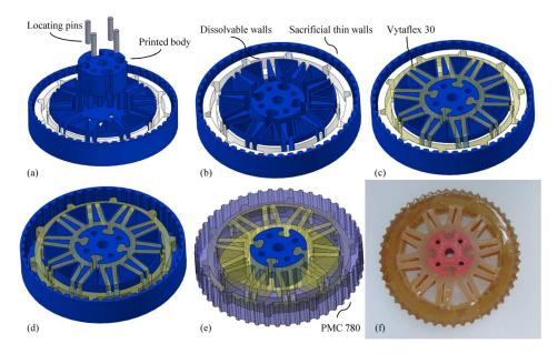
Fig. 11 Example of the airless tire, a compliant tire created with compliant spokes and a soft rim. The spokes must be anchored within the outer rim. The components are initially (*a*) printed and (*b*) assembled. (*c*) The spokes are first deposited with Vytaflex 30, and then (*d*) the dissolvable components are removed through the use of a lye bath. In the final step (*e*), the outer rim is deposited, and the outer mold features are broken apart to produce the finished wheel (*f*).
