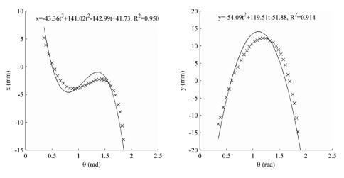
Fig. 9 Flexure joints can be approximated as revolute joints under certain operating regimes. Buckling behavior of the flexure shifts its effective center of rotation at the upper and lower limits of its driving tendon's actuation space. Mechanisms utilizing flexural joints should be designed with this behavior in mind.
