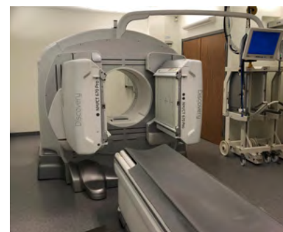
Figure 1: Example of SPECT/CT gantry and table
