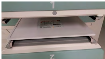
Figure 2: Implementation of extrinsic uniformity test with a ^{57}\text{Co} flat source
