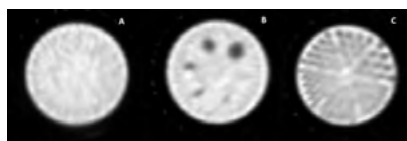
Figure 10: The Jaszczak phantom in three specific areas: homogeneous area (a), cold spheres (b) and cold bars (c).
