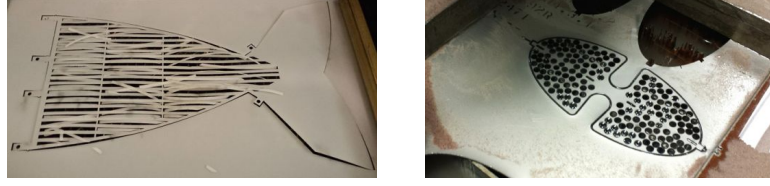
Fig. 6: Laser cut center constraint layer and water jet head constraint
