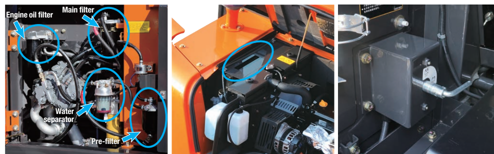
Grouped remote filters and inspection points
