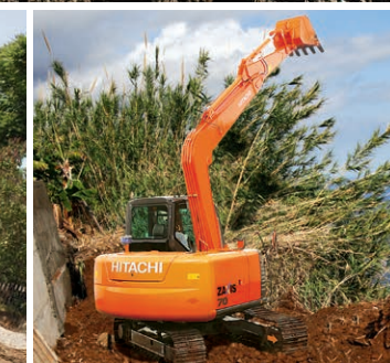
Shown equipped with an optional 4-side reinforced arm and pre-cleaner.
